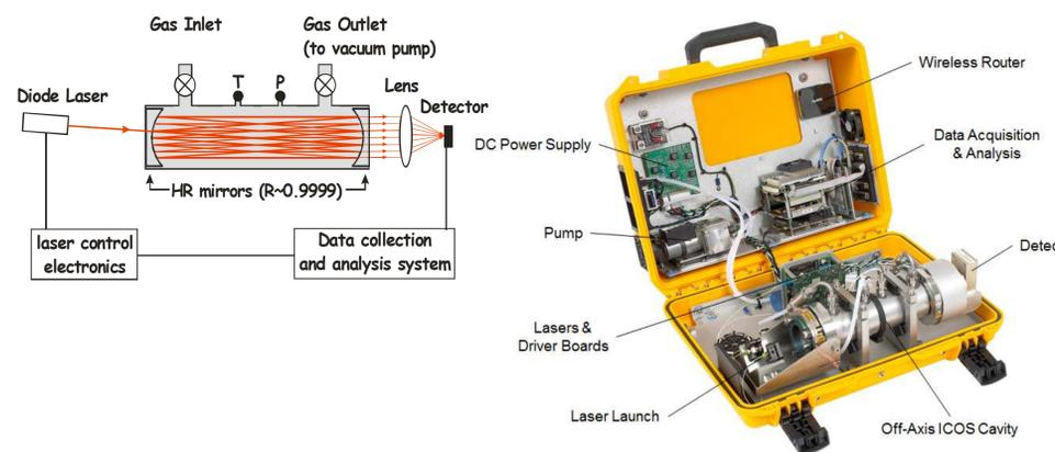
Gas measurements were recorded using LGR's Ultraportable Greenhouse Gas Analyzer (model 915-0011). (left) Schematic diagram of the optical layout of LGR's patented (Off-axis ICOS) cavity enhanced laser absorption measurement strategy ([www.LGRinc.com](http://www.LGRinc.com)). (right) LGR's Ultraportable Greenhouse Gas Analyzer (15 kg, 70 W) used to record measurements of CH<sub>4</sub> and CO<sub>2</sub> in water.
