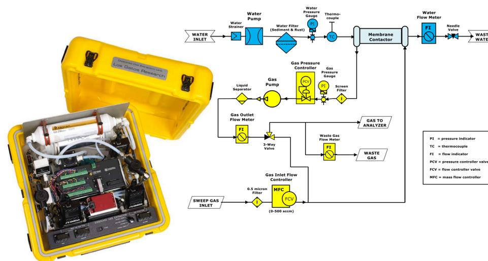
**Dissolved Gas Extraction Unit (45 W, 16 kg) controls the pressure and flow rates of sampled liquid (30-45 psia, 1-2 L/min) and sweep gas (0.15-1 L/min).**
