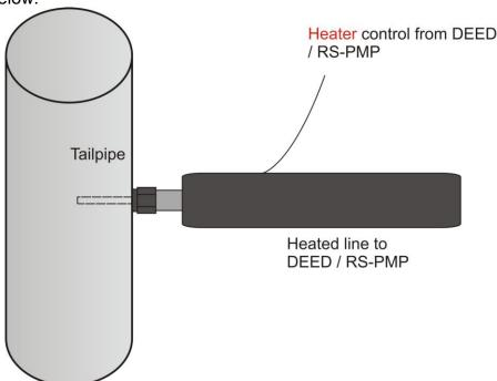
The DEED-150 is connected to the tailpipe with a 10mm Swagelok™ and uses a perforated probe to draw the sample from the tailpipe. The entire line from the tailpipe to the DEED inlet is heated to approximately 60 degrees celcius to avoid condensation of water. The heated line temperature is controlled automatically by the DEED system to optimal value. For the user there is no need to adjust any operation parameters from the DEED system when using the DEED-150 post-dpf sampler.
