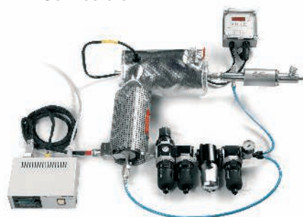
Dekati® Double Diluter setup for combustion measurements
