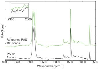
PA301 gives an equal SNR with just one scan, as opposed to 100 scans by its commercial alternative. This means that overnight measurements can be now performed in only a few minutes. A polyethene sample was analyzed with FTIR using resolution of 8 cm<sup>-1</sup>, OPD 0.16 cm/s, and using helium purge in both systems.
