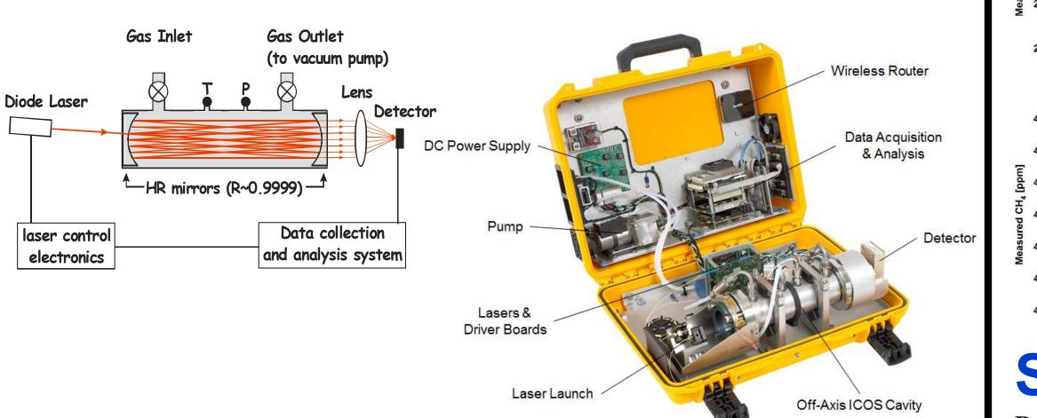
Gas measurements were recorded using LGR's Ultraportable Greenhouse Gas Analyzer (model 915-0011). (left) Schematic diagram of the optical layout of LGR's patented (Off-axis ICOS) cavity enhanced laser absorption measurement strategy (<u>www.LGRinc.com</u>). (right) LGR's Ultraportable Greenhouse Gas Analyzer (15 kg, 70 W) used to record measurements of CH<sub>4</sub> and CO<sub>2</sub> in water.
