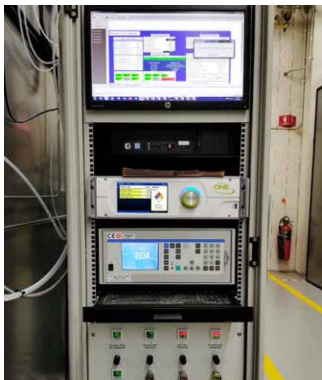
Figure 1. A US vehicle OEM has tested GASERA ONE SHED instruments against the US EPA Tier III standard and found them suitable for vehicle testing.
