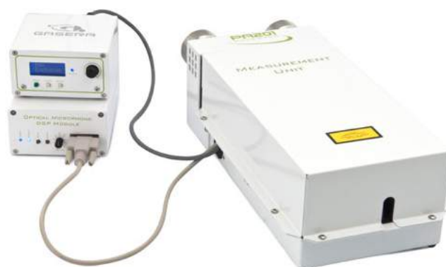
Fig 1. PA201 photoacoustic cell for research use with its gas exchange controller and DSP modules.
