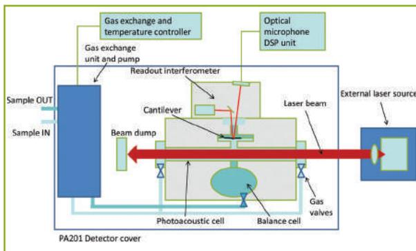
The cantilever sensor is made out of silicon which is a highly stable material and this is why the sensor is practically immune to temperature and humidity variations. Also, the sensor is not exposed to wearing.
