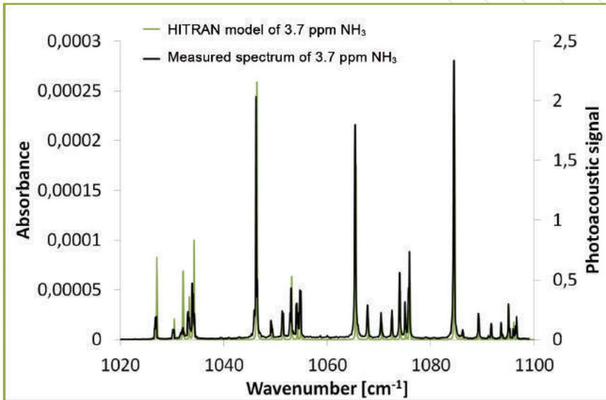
Spectrum of 3.7 ppm ammonia sample was measured using the PA201 combined with a continuous wave external cavity quantum cascade laser (CW EC QCL), which was tuned over the wavenumber range from 1020  $\text{cm}^{-1}$  to 1100  $\text{cm}^{-1}$ . Mechanical chopper was used for modulation and the maximum optical power of the laser was 62 mW.
